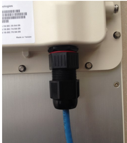
Figure 14 - Connect Ethernet cable with waterproof plug to A3-Ei
