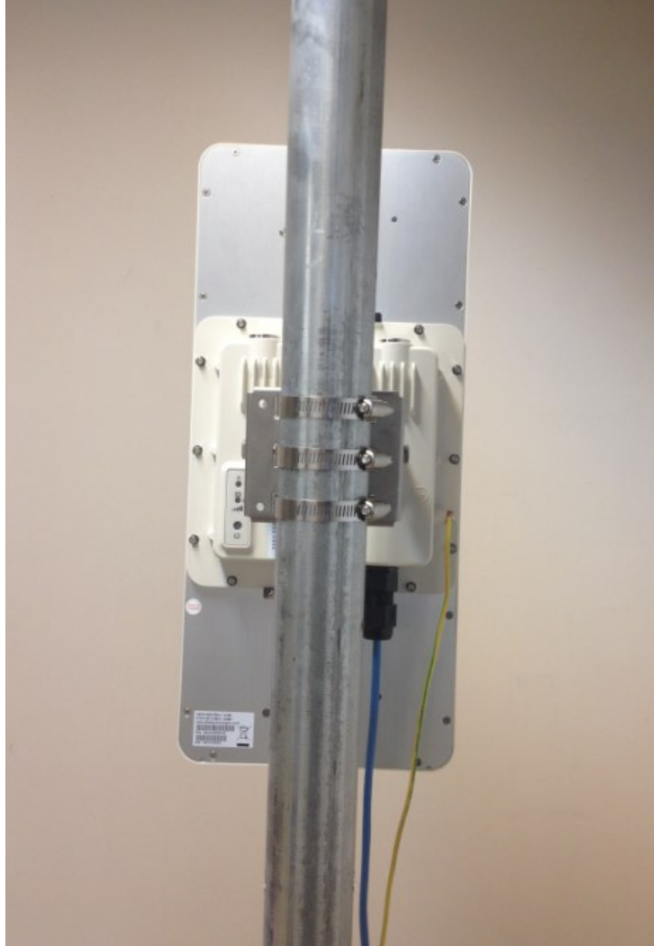
Figure 17 - Typical setup of A3-Ei on the pole
