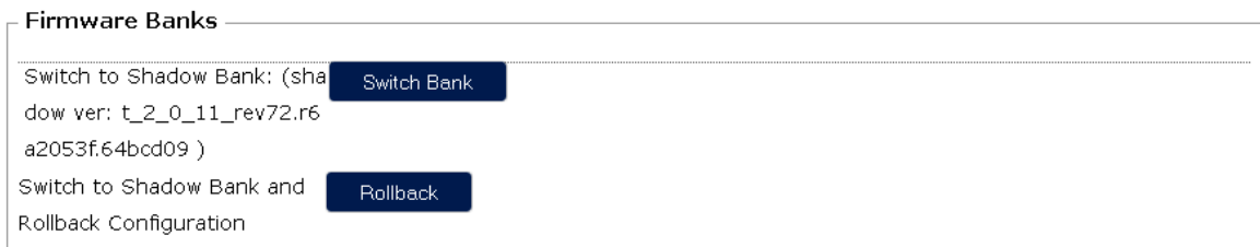
Figure 3-33: System Backup / Flash Firmware Page, Firmware Banks Section
