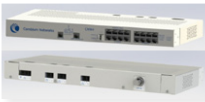
FIGURE 3. The Rack-Mounted Cluster Management Module 4
