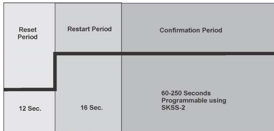
Figure 10-8 Smoke Verification Cycle
