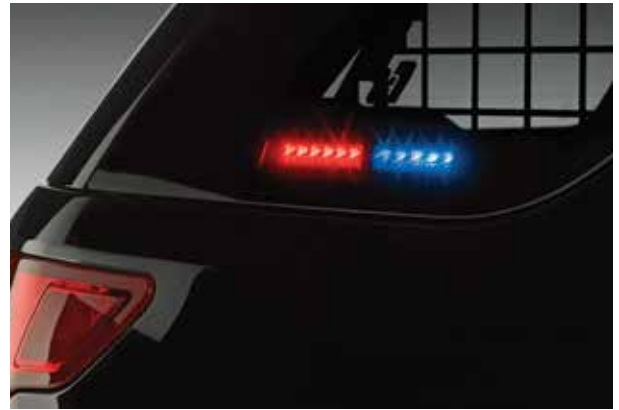
Two IPX620B-BR mounted with IPX-RSW3 bracket in rear window, on Ford Police Interceptor Utility
