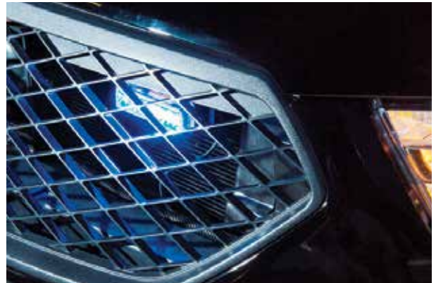
IPX620B-BR mounted with IPX-GRL5 bracket in grille, on 2013 Ford Police Interceptor Sedan
