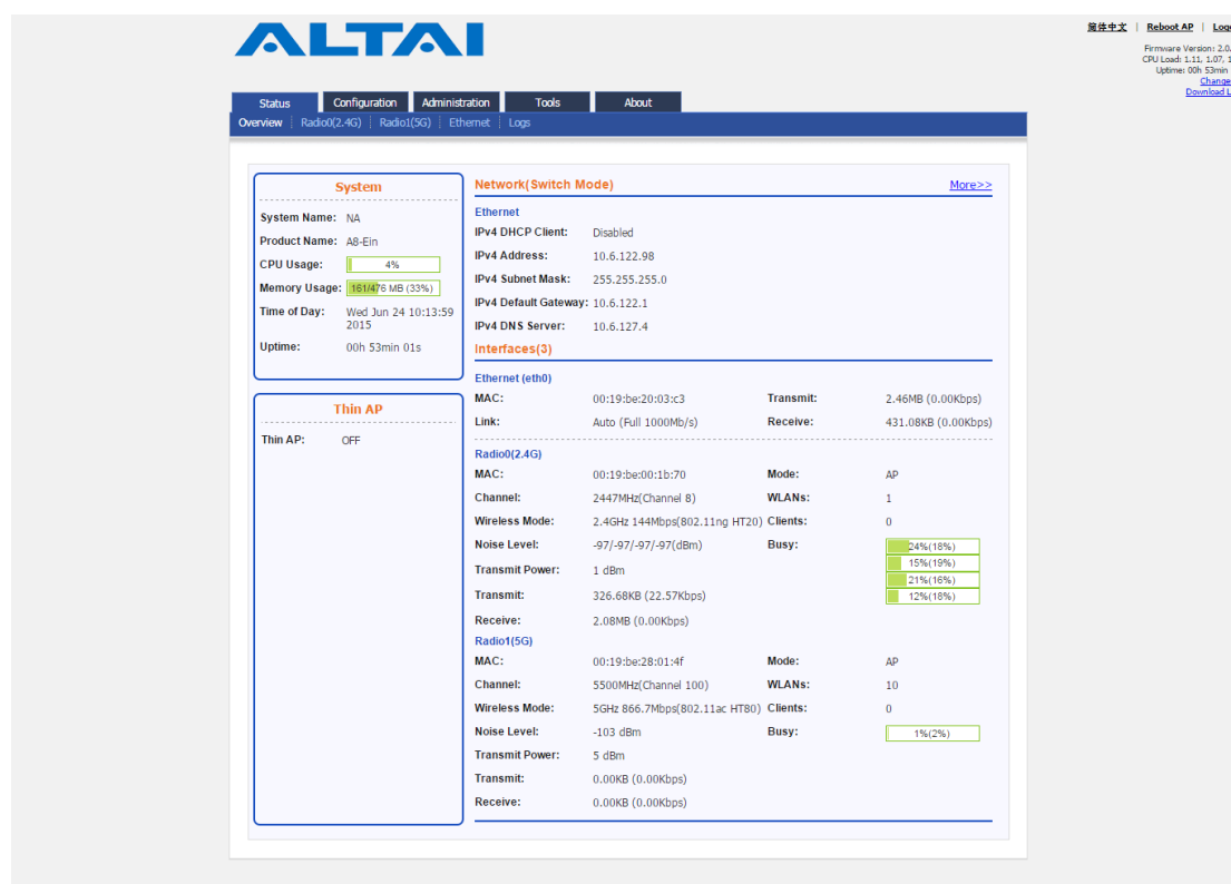
Figure 4 – AP Status Overview
