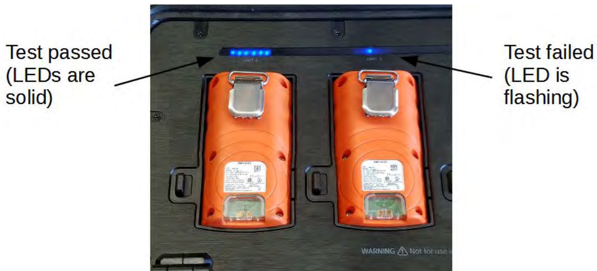
Figure 4–1 LED pattern indicates test pass or fail
