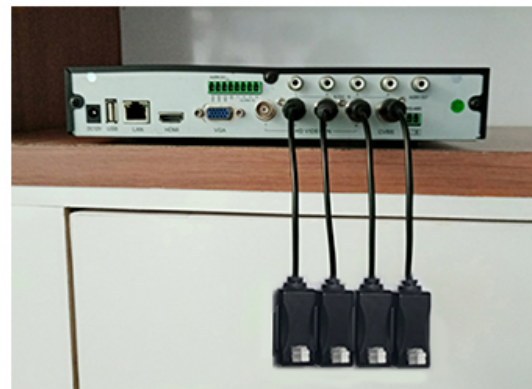
Baluns click together for a neat installation
