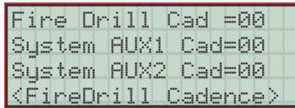
Figure 7-16 Special Cadence Patterns for Fire Drill and Auxiliary Alarm Events
