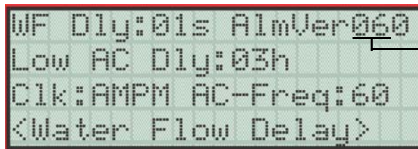
Figure 7-17 Water Flow Delay Programming Screen
