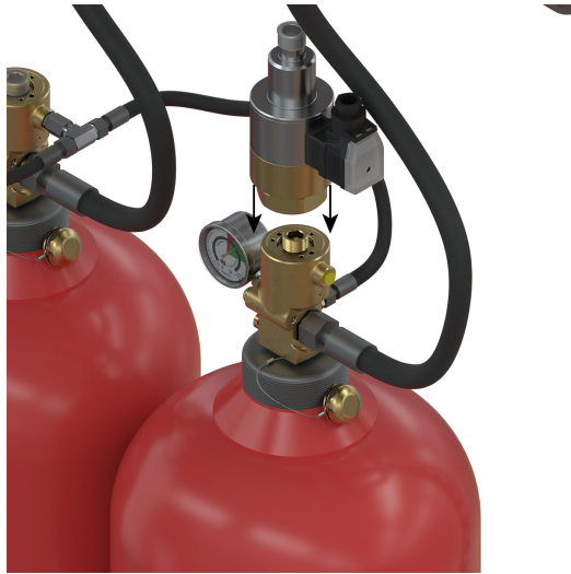
Figure 6.22: Install releasing solenoid to primary valve
