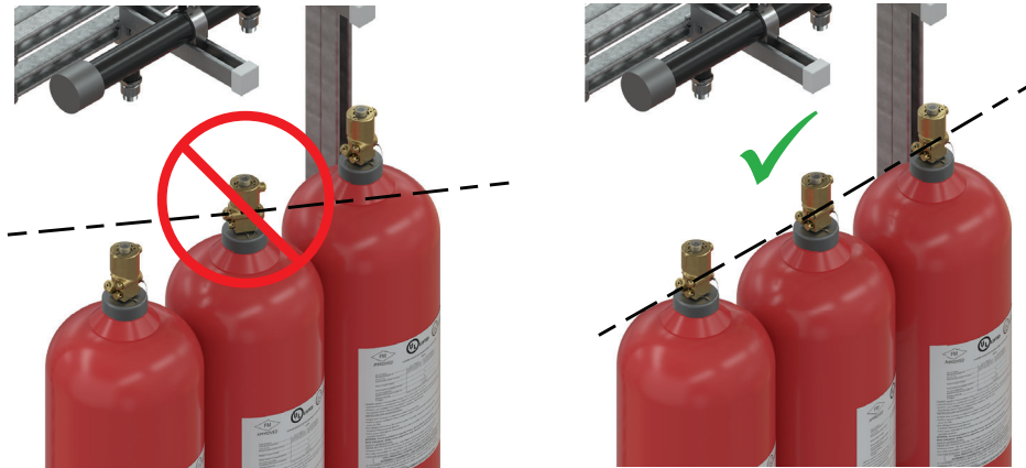
Figure 6.6: Align valve with manifold
