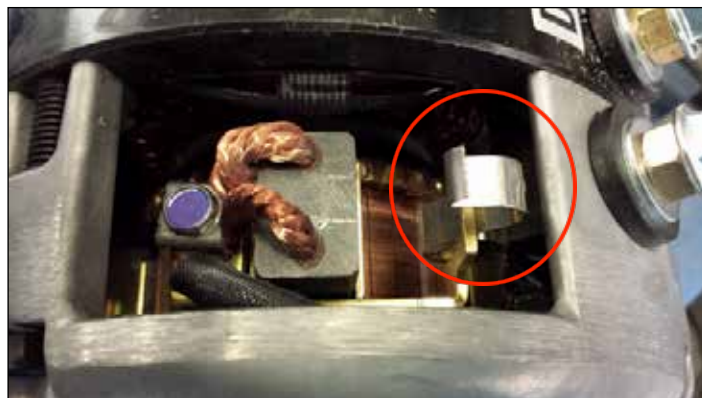
Figure 10 Brush Spring Latched on Post
