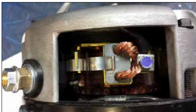
Figure 17 Placing the Brush Spring
